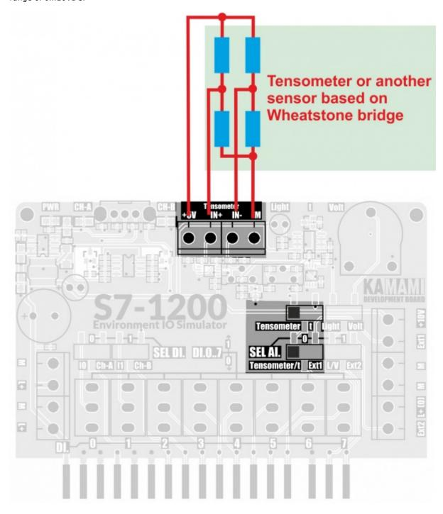
Tensometer or other sensor with differential output should be connected to the IN + and IN- terminals and + 5V and M supply lines.
