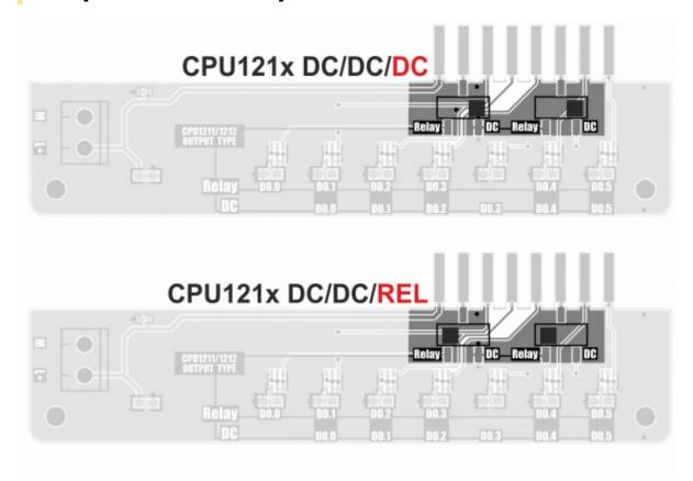
Depending on the state of the selectors installed on the output board, its configurations can be adapted to PLCs with transistor (DC / DC ) or relay (DC / DC / REL) outputs.
