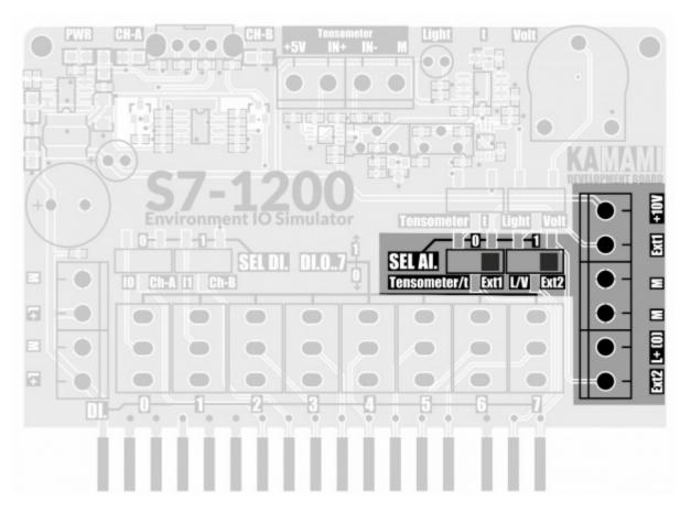
The Ext1 and Ext2 inputs are not equipped with conditioners, the voltages are fed directly to the PLC analog inputs:
