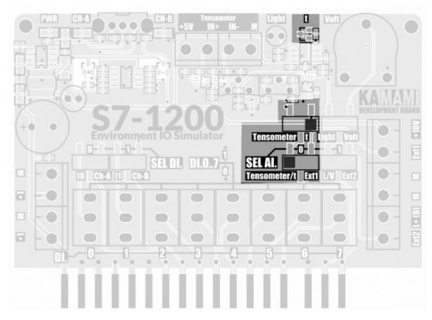
On the input board there is a temperature sensor with analog output (MCP9700AT-E/TT with 10V/V amplifier). The amplifier output voltage for the measuring range +5...+105°C is in the range of 0...10VDC.
