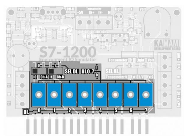
The KA-LOGOS71200-IO-Simulator board is equipped with toggle switches marked DI.0..DI7, setting the selected digital state "0" or "1" on individual digital inputs DI.x of the PLC controller.
