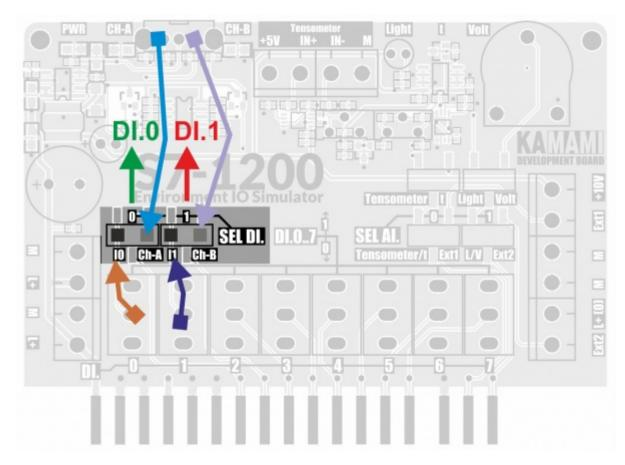
SEL DI.0 and SEL DI.1 selectors are used to connect DI.0 and DI.1 toggle switches DI.0 and DI.1 or encoder outputs - respectively:
