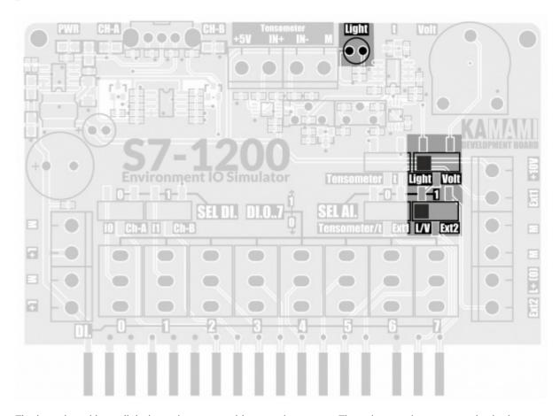
The input board has a light intensity sensor with an analog output. The voltage at its output varies in the range of  $0 \dots + 10$ VDC, its value increases as the light intensity on the sensor increases.
