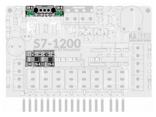
The input board is equipped with a two-phase AB encoder, which via the forming system (Schmitt trigger) provides signals to the PLC inputs:
