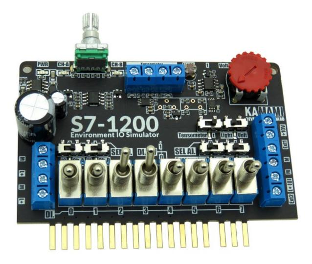
• **output** with LED diodes that allows to monitor outputs of PLC (family Siemens S7-1200). Diodes are driven by Nexperia LED drivers that makes sure all diodes are supplied with constant current, apart from input voltage fluctuations.
