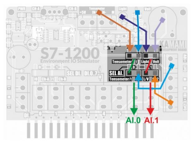
The SEL Al.0 and SEL Al.1 selectors are used to select the signal source fed to the Al inputs:
