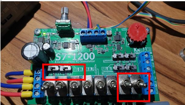
2.2. Flip each switch DI.0...DI.5 on-off-on and check if LED on the output plate DO.0...DO.5 and the green LEDs embedded in the S7-1200 controller light up (both input and output lines)
