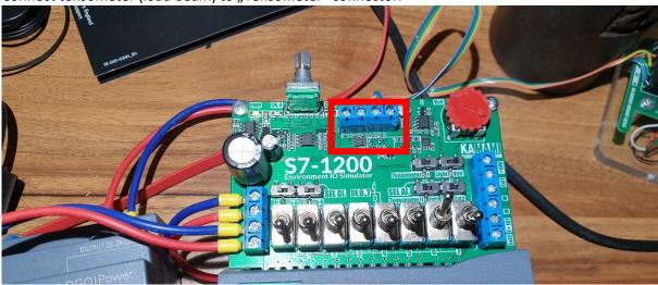
4.3. The SEL AI.0 switch should be set to the "Tensometer/t" position.
