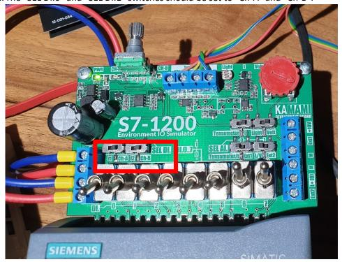
5.3. Turning the encoder knob we observe the LED DO.0...DO.5, which should turn on sequentially:
