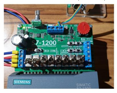
1.2. The controller outputs should be connected to the output board, the switches located in its upper right should be in the "DC" position.
