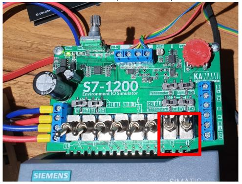
5.2. The "SEL DI.0" and "SEL DI.1" switches should be set to "Ch-A" and "Ch-B".
