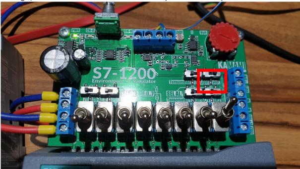
3.6. By turning the red knob of the "Volt" potentiometer we check if the statuses of the DO.0...DO.5 outputs change, with the potentiometer knob being closer to the rightmost position of the "Volt" potentiometer, the higher DO.x LED will light up.
