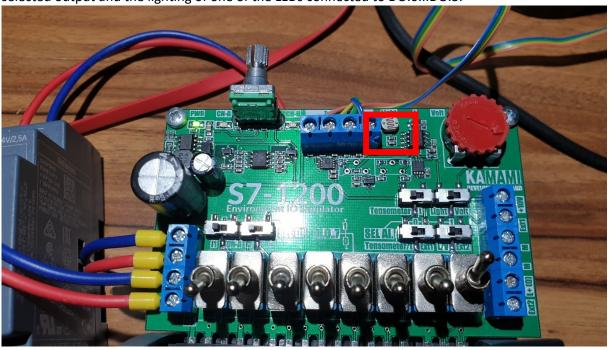
3.5. The "Light/Volt" switch should be now set to the "Volt" position - as in the photo below.
