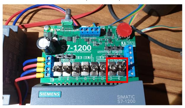
3.2. The SEL Al.1 switch should be set to the "L/V" position.
