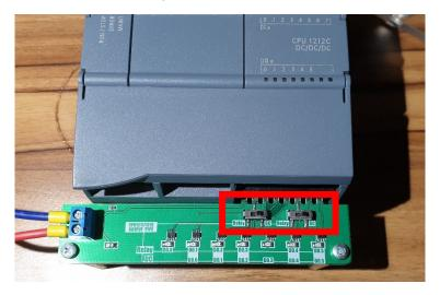
1.3. The power supply terminals of both boards should be connected to each other and connected to the 24VDC power supply. When the set is properly powered, the "PWR" LED located in the upper-left corner of the (large) input board will light up - as in the photo below.
