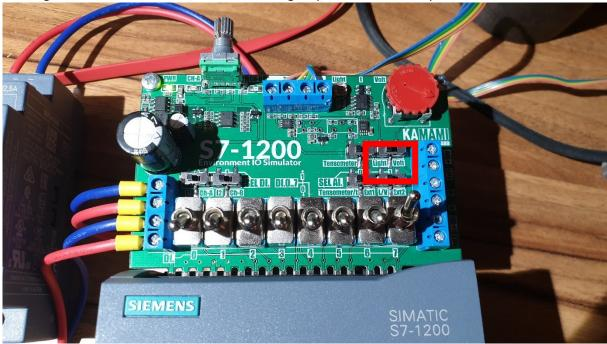
3.4. The light sensor marked on the board as "Light" should be illuminated or shielded from light, which - depending on the intensity of light falling on the sensor - changes the state of the selected output and the lighting of one of the LEDs connected to DO.0...DO.5.
