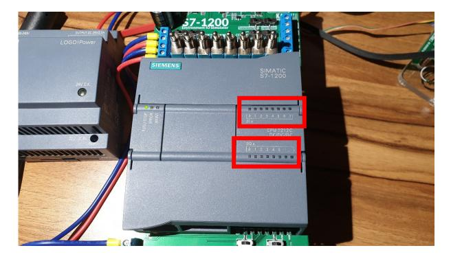
2.3. Passing test # 1 requires the reaction of the respective outputs to state changes on all inputs.
